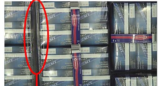
The two products are the same in the left and right image (4-pack wrap, same bar code). The difference emerges from the caddie preparation: half caddies (right image) preparation requires additional plastic wrapping (circled in red). ViDi green locks onto this “soft feature” by itself and reliably detects it across images tolerating significant variation in appearance.
